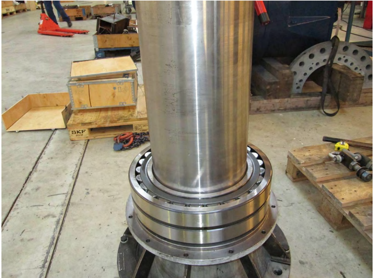
Bearing exchange main bearing.
