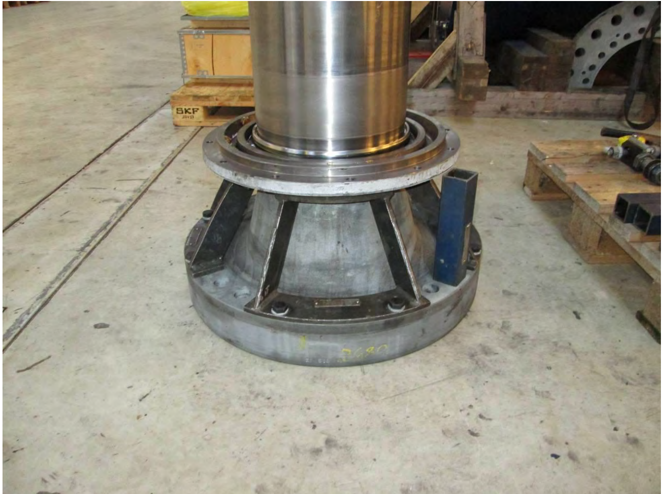
Bearing exchange main bearing.
