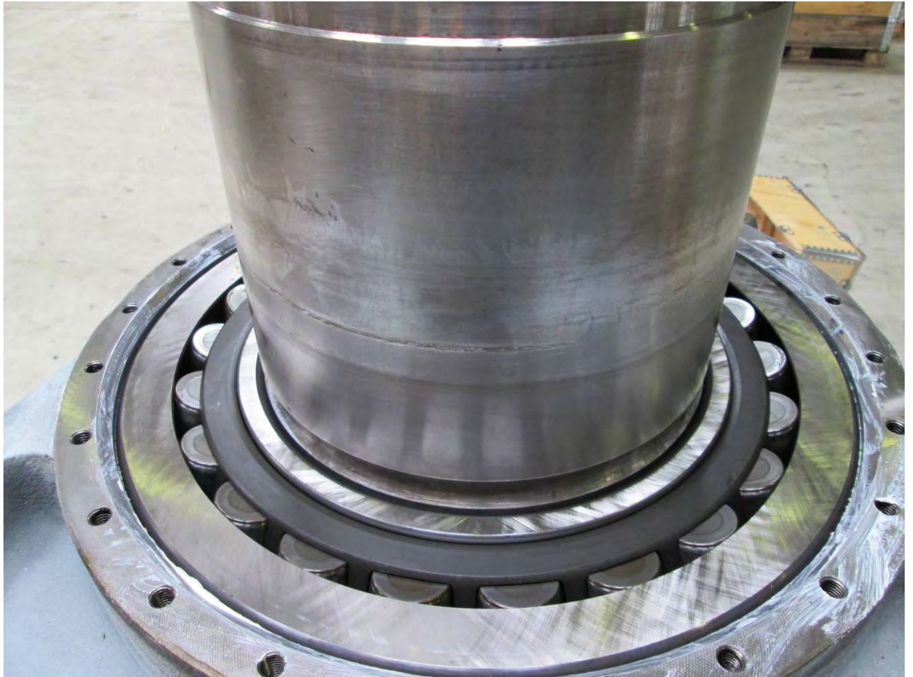
Bearing exchange main bearing.
